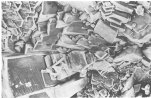
Figure 5 Manganese phosphate crystals on rough abraded surface.*
