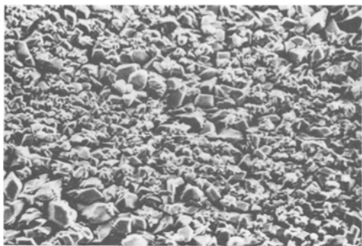
Figure 9 Manganese phosphate deposit on low reactivity polished surface.†
