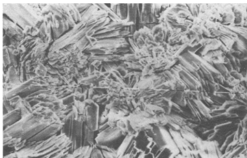
Figure 10 Fracture of crystals caused by heating.†
