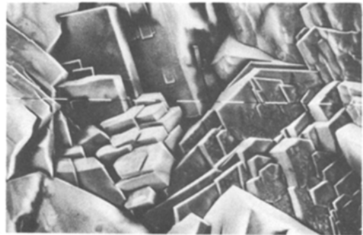
Figure 7 Manganese phosphate crystals deposit from impurity nuclei.*
