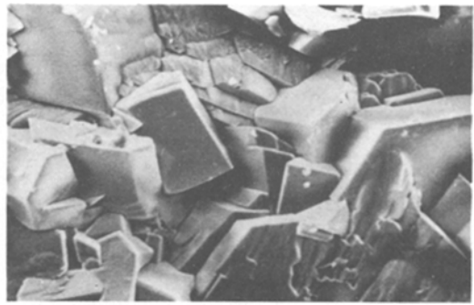
Figure 6 Manganese phosphate crystals on acid pickled abraded surface.*
